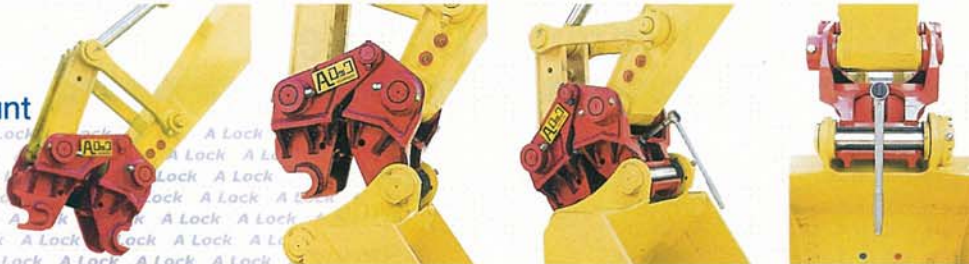
Hook the arm side claw of the A Lock onto the pin of the attachment.
